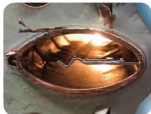
Pickled exchanger with 1,5% FERRONEX in 3 hours
