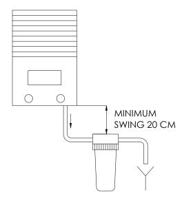
The filter must have at least 20 cm of leaf against the discharge point of the boiler
